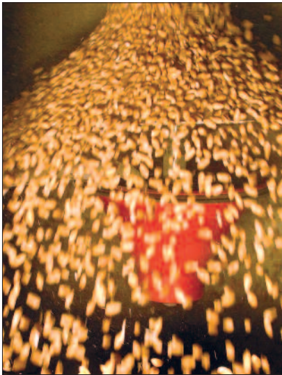
Figure 6. Motion of seeds in the dressing chamber
