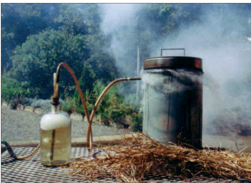
Figure 2: Apparatus for producing smoke-saturated water
