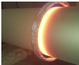
Figure 2 Inductive remelting process of the NiCrBSi coating
