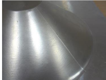
Figure 16 Final part made with TSISF
