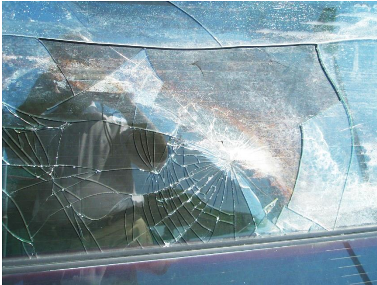
Figure 10. Broken PV amorphous PV panel (2010) 14
