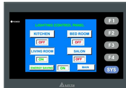
Figure 10 Lighting control panel
