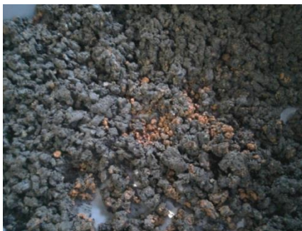
Figure 3 Sludge mashed through a sieve (No. 5)
