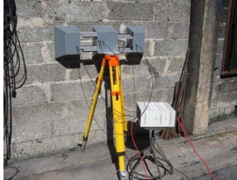
Figure 2 M-sequence UWB radar system
