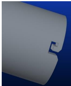
Figure 15. Upper body connecting slot
