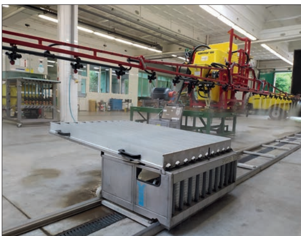
Figure 1: PESSL Sprayertest 1000 mobile spray scanner for the measurement of the transverse distribution uniformity of a horizontal boom sprayer
