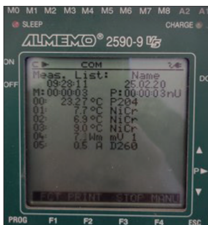
Figure 1: Almemo data logger 2590-9 and temperature sensor NiCr-Ni type.
