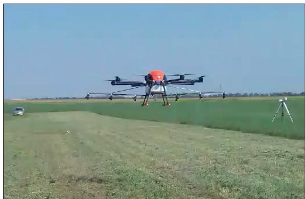
Figure 5: Work quality inspection of spraying drone
