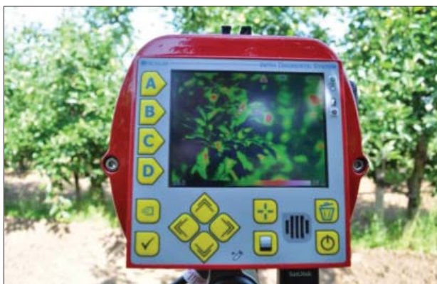
Figure 1: HEXIUM PYROLATER-12 thermographic camera and its image in an orchard
