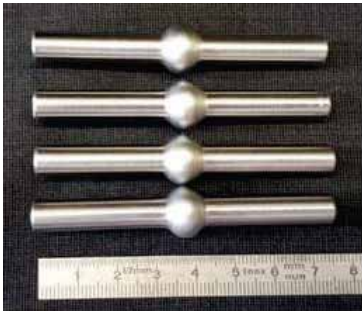
Fig. 3. Test specimens after a SICO test
