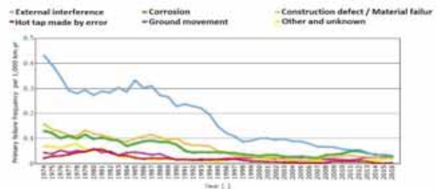
Figure 4. Failure frequencies of different causes by EGIG [7]
