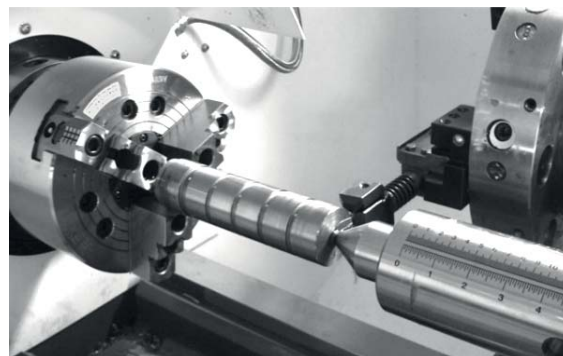
Figure 1. Executing of burnishing process
