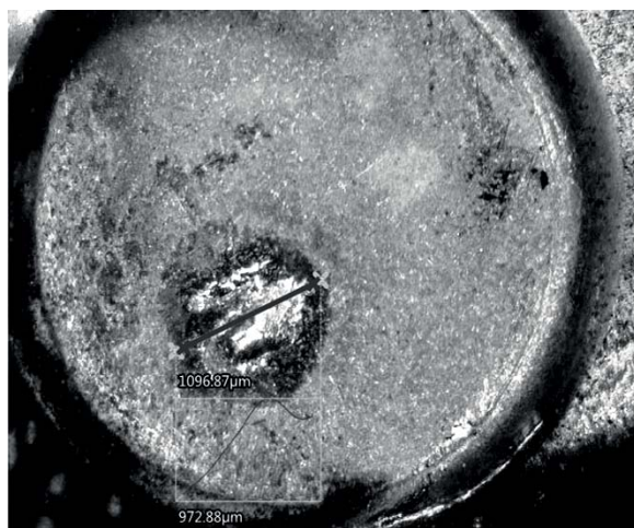
Figure 4. Contacting surface of a micro switch (Type K2)
