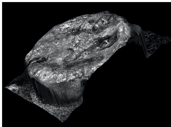
Figure 3. Contacting surface of a micro switch (Type D1)
