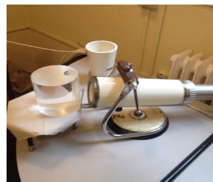
Figure 1: Thyroid measurement: detector, shielding and neck phantom
