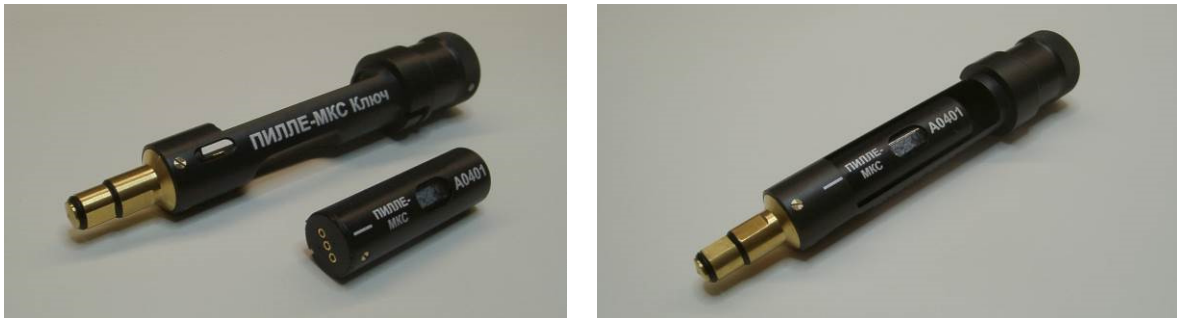
Figure 2: The new Pille dosimeters (left: universal key and the dosimeter unit, right: the dosimeter inserted in the universal key).
