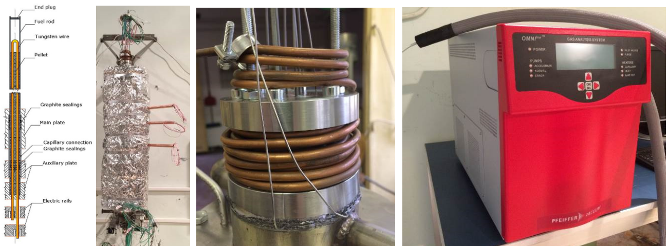
Figure 1: new elements of the CODEX facility (left-to-right) scheme of the heated fuel rod, view of the bundle with thermal insulation, cooler of the test section and mass spectrometer
