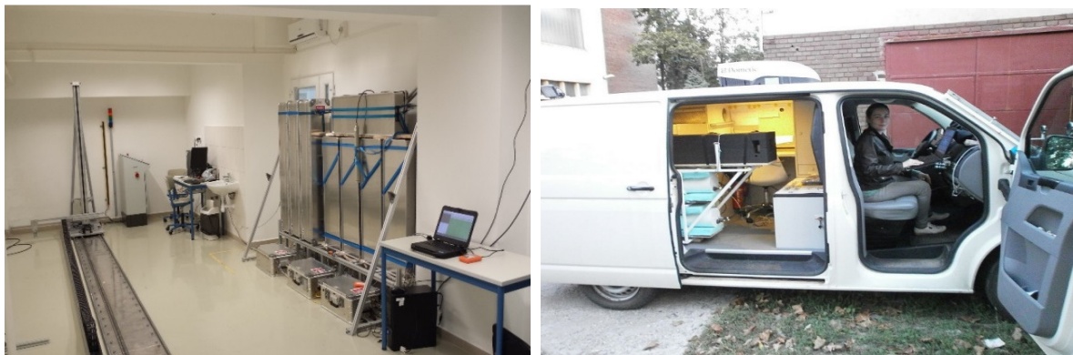
Figure 2: Relocatable and mobile radiation detector modules of Symetrica under test in the test laboratory (left) and in the mobile laboratory (right) of MTA EK
