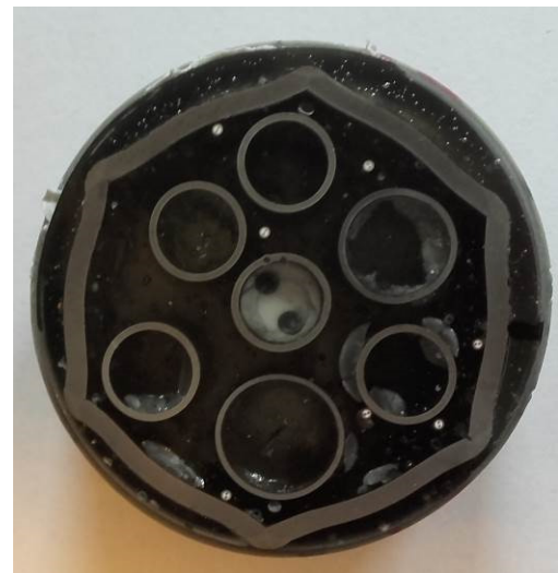
Figure 1: Maximum cladding temperatures in the CODEX-LOCA-SFP1 and CODEX-LOCA-SFP2 tests (left) and cross section of CODEX-LOCA-SFP2 bundle at 480 mm elevation (right)
