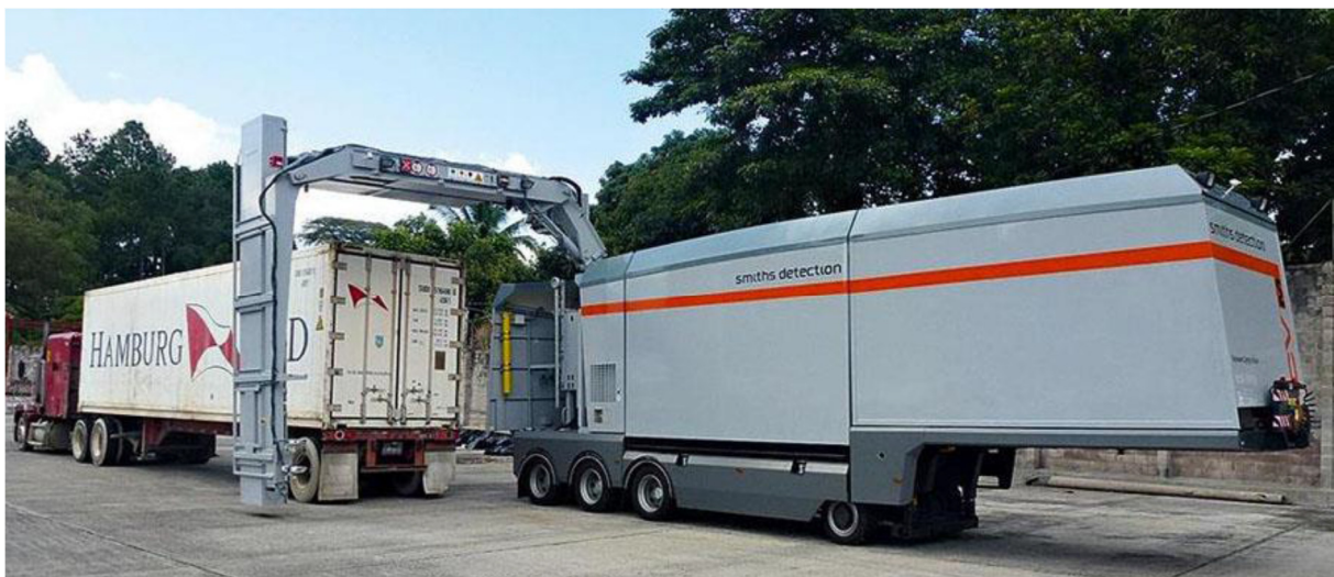
Figure 1: The HCVM-T X-ray scanning system with the pass through mode deployed.
