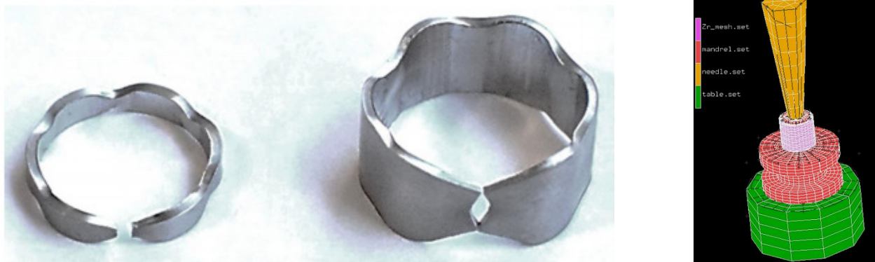
Figure 3: View of 2 mm and 8 mm long ductile cladding rings after mandrel tests (left) and finite element model of the segmented tool
