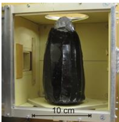
Figure 1: An obsidian core in the sample holder of the Budapest NIPS station
