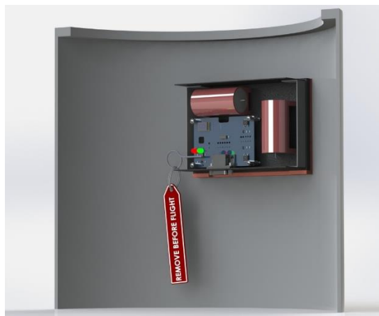
Figure 1: The two GM counters and their electronic unit mounted onto the REXUS rocket module (REM-RED)
