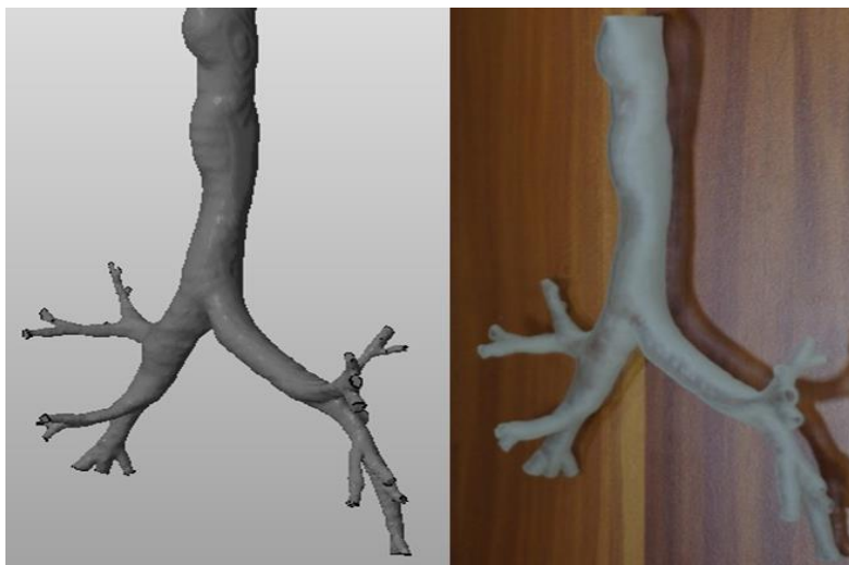
Figure 1: Reconstructed digital (left side) and physical, printed out, (right side) geometries of the central airways
