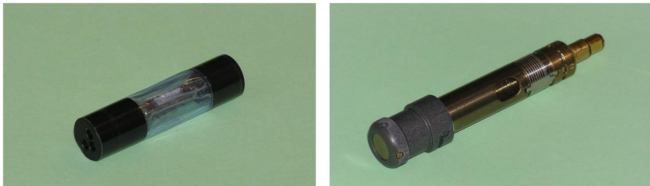
Figure 1: Prototype of the new Pille dosimeters dedicated to EVA measurements: dosimeter "cartridge" of reduced shielding (left) and its read-out socket (right)
