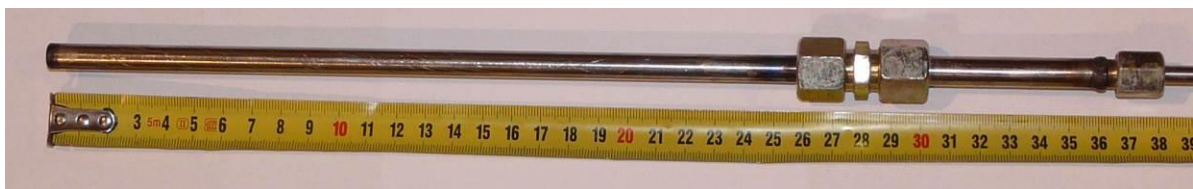
Figure 2: View of the cladding sample for secondary hydriding test
