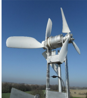
Figure 5.: Unconventional WTs: Dual-Rotor Wind Turbine
