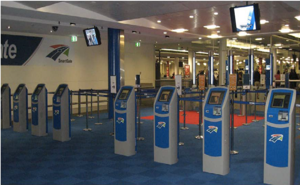
Figure 1: Photo of Smart Gates (Facial and Fingerprint) Brisbane International Airport from Frontex, 2010.
