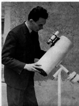
The author and his 6-inch rich-field reflector. Only 18½ inches in focal length, it gives a wide, bright field. Many deep-sky objects have been observed with it, despite city lights. The 5x finder has an aperture of 1½ inches. Like most mountings built by Hungarian amateurs, this equatorial is made of simple pipe fittings because of their availability. Mr. Szentmártoni plans to replace this mounting with one of the new type. The mirror was aluminized in Budapest, and a prism was selected at the Newtonian diagonal, since small flat mirrors are not on the market there.
