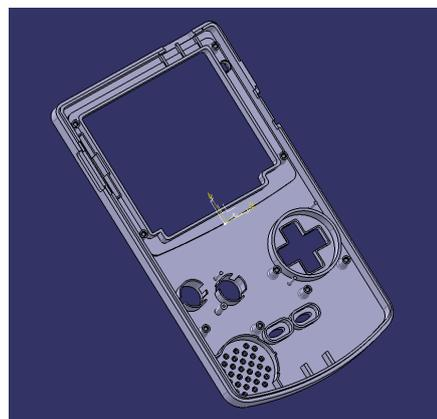
Figure 1: CAD model of the shell of a handheld game console.
