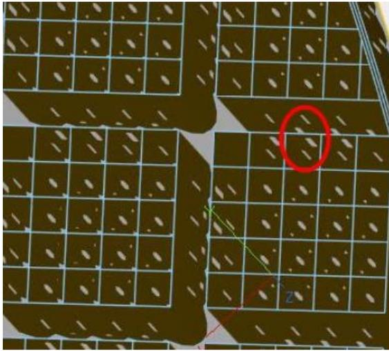
Figure 12: “Fragmentation” and lightening of the diamond shape highlighted by a red circle
