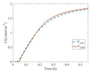
Figure 15: Step response of the system with CFD methods and CM
