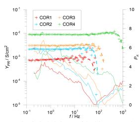
*Figure 8:* Principal admittance of the COR system calculated by Eq. 4 using Method (i) (points) and Method (ii) (dotted lines). Solid lines indicate the  $P_R$  values obtained using Method(ii).
