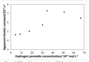
*Figure 6*: Effect of the concentration of  $H_2O_2$  on the apparent rate constant of RhB photodegradation in the absence of NPs. Experimental conditions: concentration of RhB is  $1.8 \times 10^{-5}$  mol/L, initial pH is 7.5, and irradiation time is 140 mins.
