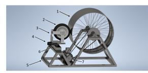
*Figure 7:* The CAD model of the apparatus: 1. drum using different modelled road surfaces, 2. test wheel, 3. test wheel mounted on load cells, 4. linear stage for moving the test wheel towards the drum, 5. frame, 6. linear stage for lowering the test wheel onto different surfaces, 7. AC motor driving the drum.
