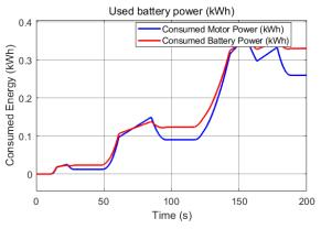
Figure 21: Energy consumption of the motor and battery
