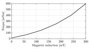
*Figure 6:* Measurement example of the MR clutch. The transmitted torque of the clutch at a constant speed as a function of the magnetic induction.
