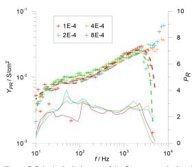
*Figure 7:* Principal admittance of the Cu system calculated by Eq. 4 using Method (i) (points) and Method (ii) (dotted lines). Solid lines indicate the  $P_R$  values obtained using Method(ii).
