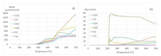
Figure 3: Evolution of molar quantity a) and weight percentage b) as a function of temperature
