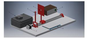
*Figure 9:* Measuring the ultrasonic distance. The device consisted of a fixed ultrasonic transmitter (2) and a receiver (3) moved by a linear stage driven by a stepper motor (5). The control system and circuit (1) as well as the power distribution and power supply system (4) were located in separate boxes. A 7-inch display was installed on the device (6).
