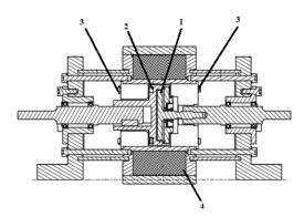
*Figure 5:* Schematic diagram of the magnetorheological clutch. The magnetorheological fluid was located between the input (1) and output (2) disks. The input disk was connected to the shaft by a ball bearing. The clutch was sealed by an O-ring at the output disk and an oil seal at the ball bearing. A coil (4) consisting of approximately 1200 turns of copper wire was located around the disks. The magnetic field lines were directed through the fluid with the help of magnetic flux guiders (4).
