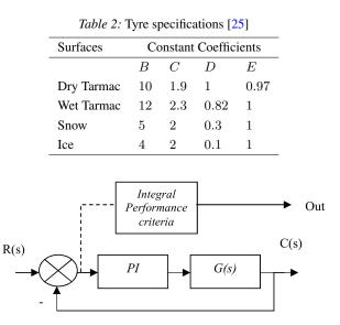
Figure 5: Control loop by applying a PI Controller
