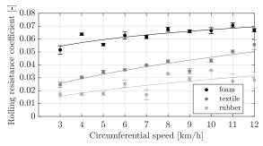
*Figure 8:* The rolling resistance coefficient measured on the three modelled road surfaces.
