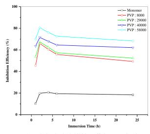
*Figure 3:* Variation in the inhibition efficiency against immersion time for carbon steel at various molecular weights of inhibition in a 1 M HClO<sub>4</sub> solution.
