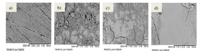
*Figure 4:* SEM images of carbon steel (a) before immersion, (b) after immersion in the acidic solution (1 M HClO<sub>4</sub>) in the absence of inhibitors, (c) after immersion in the acidic solution containing  $5 \times 10^{-3}$  M PVP58000, and (d): (c) + KI.
