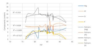
*Figure 5:* Effect of Mg, Al, Si and K constituents on Vickers hardness
