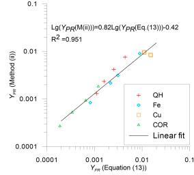
*Figure 9:* Correlation between the logarithms of the principal admittance obtained by Method(ii) using Eqs. 4 and 13 in Ref. [37]. The linear fit was calculated from the logarithms of the principal admittance data. The QH (quinhydrone) data were taken from Ref. [36].
