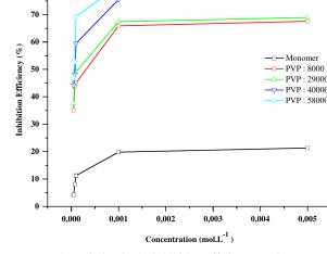
*Figure 2:* Variation in the inhibition efficiency against concentration in a 1 M HClO<sub>4</sub> solution, using various molecular weights of the inhibitor.
