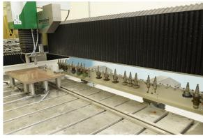
Figure 1: The CNC equipment and various tools
