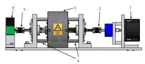
*Figure 4:* Demonstration device of a magnetorheological clutch. Our magnetorheological device uses an induction motor (1) as a torque source driven by a VFD, moreover, both the driver and driven parts are connected by a flexible coupling (2, 5) to the actual clutch (3). The clutch is held in place by slotted placeholders (4).
