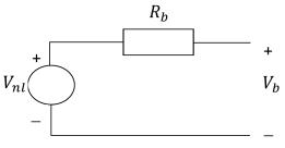
Figure 10: Battery equivalent circuit model
