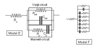
*Figure 2:* Model E by applying the general scheme and Model F with the series of Maxwell circuits connected in parallel.
