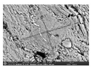
Figure 3: Imprint of the 136° square-based diamond pyramid
