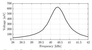
*Figure 10:* Example measurement made by the ultrasonic sensor demonstration device. The example shows the resonance curves of both the transmitter and receiver.
