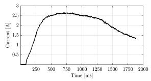
*Figure 3:* Measurement example of the induction motor drivetrain. The example presents the starting current of the motor as a function of time using frequency converters.
