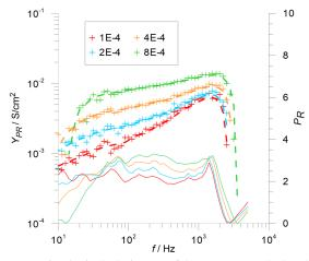
*Figure 6:* Principal admittance of the Fe system calculated by Eq. 4 using Method (i) (points) and Method (ii) (dotted lines). Solid lines indicate the  $P_R$  values obtained using Method (ii).
