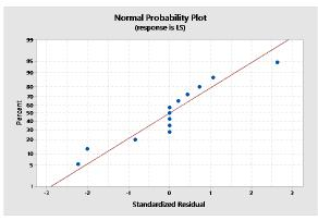
*Figure 2:* Normal probability plot of the residual plot for linear shrinkage (LS).
