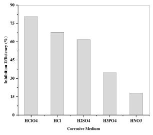
*Figure 1:* Variation in inhibition efficiency of carbon steel in different acid media (PVP:  $58,000 \text{ g mol}^{-1}$  with  $1.0 \times 10^{-3} \text{ mol L}^{-1}$  of acid medium for 2 h at 303 K).
