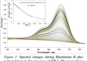
todegradation in the presence of NP-3. The inset shows the absorbance vs. time plot at 554 nm. Experimental conditions: concentration of RhB is  $1.8 \times 10^{-5}$  mol/L, concentration of H<sub>2</sub>O<sub>2</sub> is  $1.8 \times 10^{-1}$  mol/L, concentration of NP-3 is 400 mg/L, initial pH is = 7.5, and irradiation time is 140 mins.
