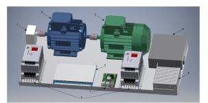
*Figure 2:* Demonstration device of an induction motor drivetrain. One two-pole (2) and one four-pole (3) induction motor were connected with flexible couplings. The motors were driven by frequency converters (8). A small DC motor was used as a tachogenerator (1). The power distribution network and control circuit were placed in a plastic box (4). The Raspberry Pi microcomputer (7) had a separate power supply (6) and was connected to a 7-inch display (5).
