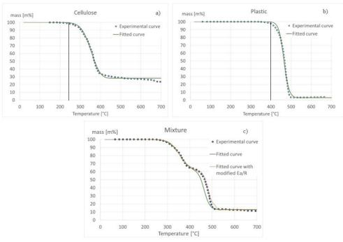
*Figure 2:* Measured [8] and simulated results using the identified parameters: a) cellulose, b) plastic, c) cellulose and plastic 50 - 50% mixture; o Experimental curve, — Fitted curve, — Fitted curve with modified  $E_a/R$ , — degradation start
