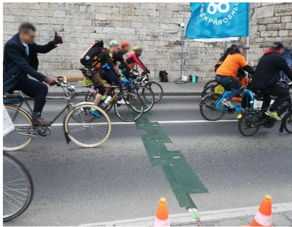
Figure 4.6 Sensor strip (covered with red adhesive tape) across a bicycle lane
