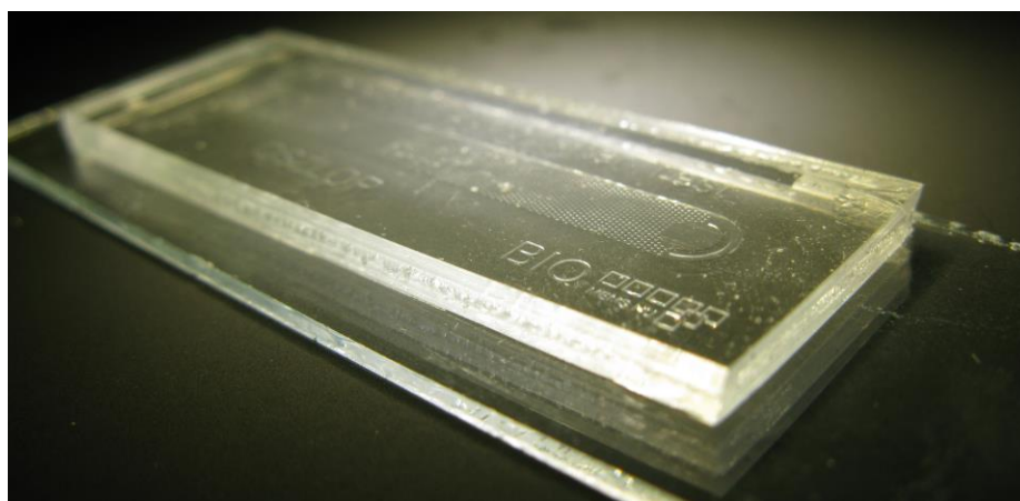
Figure 2-1. Microfluidic cartridge for testing of autonomous sample transport and preparation.
