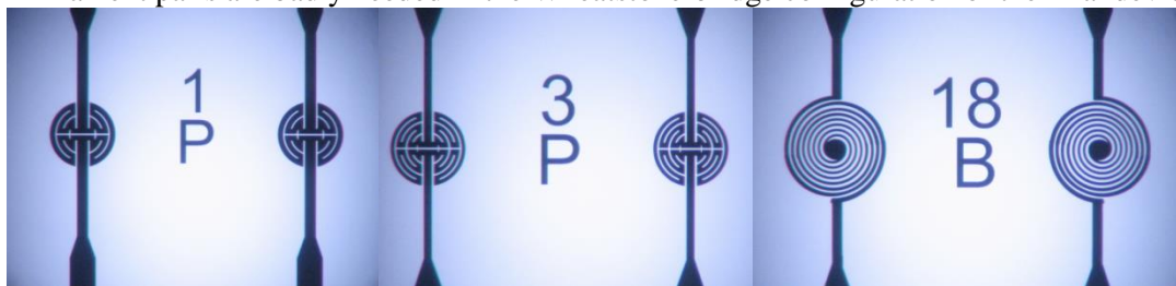
Fig. 1. Mask images of selected filament geometries for formation of uniform temperature hotplates.
