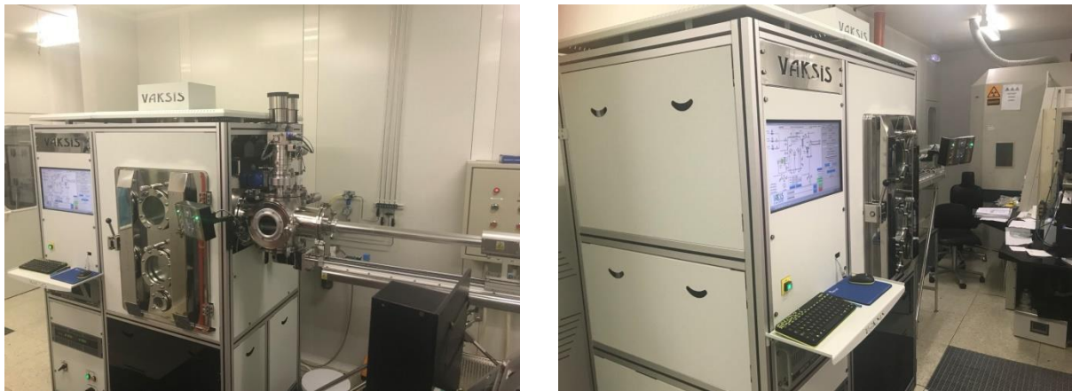
Figure 1 The VAKSIS sputtering system in operation in the clean-room of the Lab (building 29.b)
