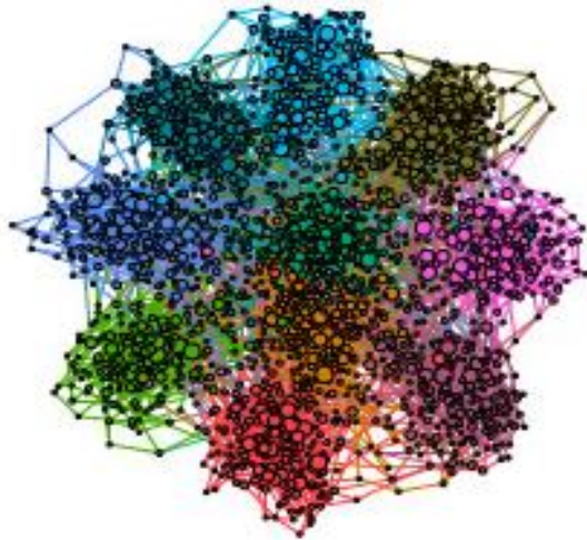
Figure 1. Example a of modular structure. Networks with 100 modules of same size of 200 nodes and number of inter-modular connections k = 10 , representing loosely and densely connected modular graphs, respectively. The network degree distribution is given by P(k) \sim k^{-2.7} . Connected modular structures can clearly be observed.
