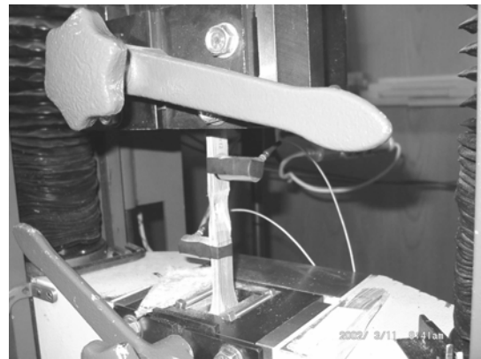
Figure 2. Fastening the transducers on the specimen with rubber bands
