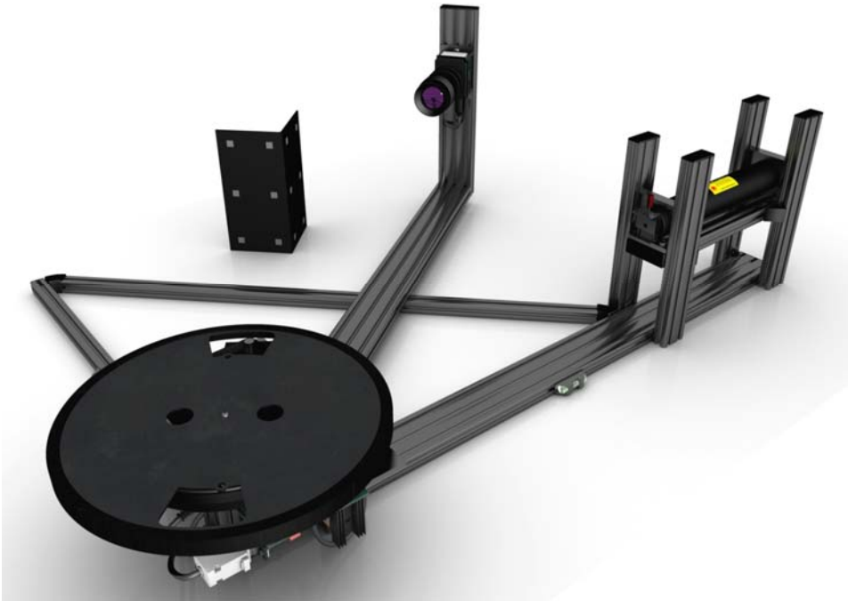
Figure 1. The active triangulation scanner with the rotating table.
