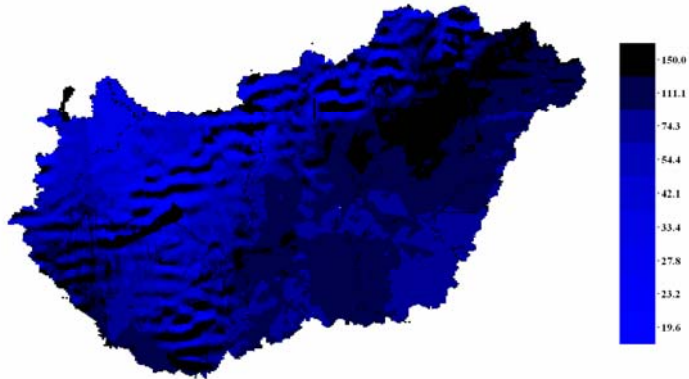
Figure 6: Payback period (in years) of the wind power plant described in the text as a function of geographical location inside Hungary.
