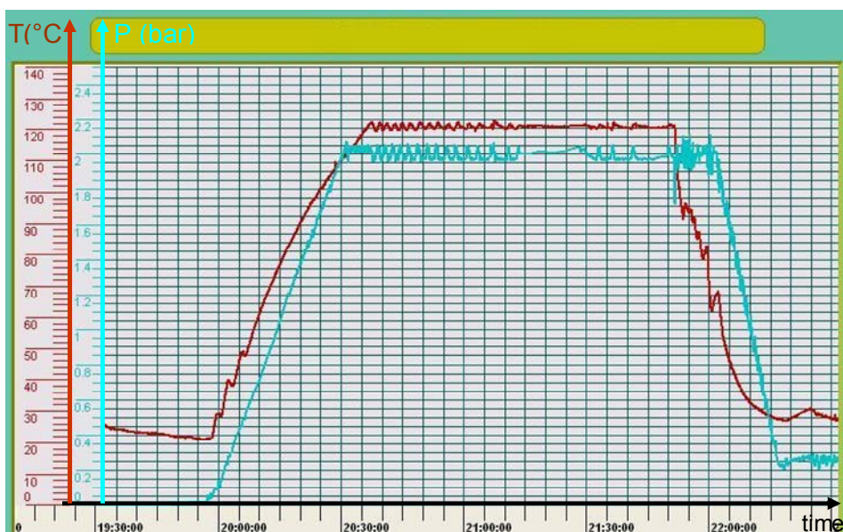
Figure 6: Insufficient steam supply
