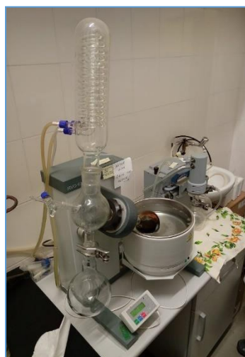
Figure 8. The single-stage rotary evaporator for distillation [8]
