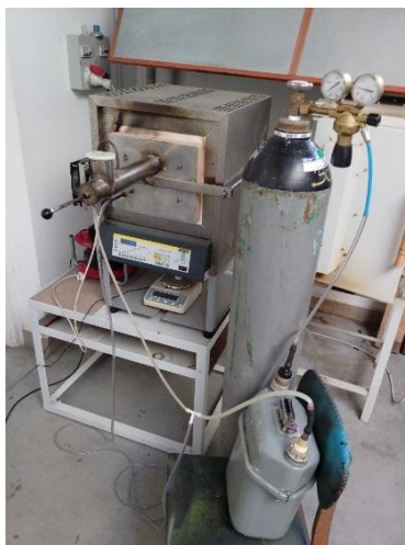
Figure 4. The improvised furnace for the torrefaction process
