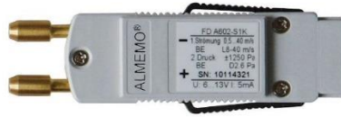
Figure 6. Differential pressure sensor
