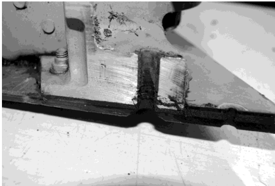
Picture 19. Aluminum and carbon fibre assembly [7]
