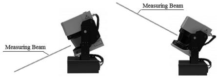
Picture 1. Laser Scanner bending mechanism. [1]
