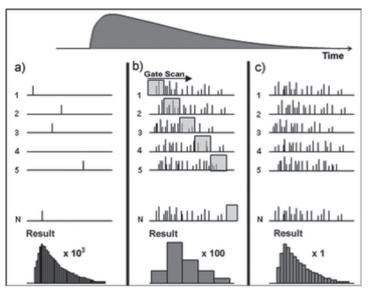
Figure 4. Various techniques for single photon counting. [5]
