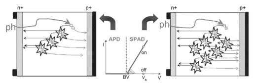
Figure 6. APDs are biased just below VB in order to have a non-diverging multiplication process (linear multiplication) of the photo-generated carriers (left side).
