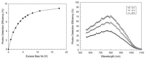
*Figure 7.* Photon-detection efficiency at different excess bias for a thin SPAD ( $W = 1 \mu m$ ) at  $\lambda = 850$  nm (left) and for a thick SPAD ( $W=25 \mu m$ ) (right). [4] [16]
