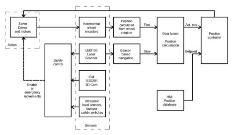
Figure 6. The block diagram of the advertising mobile robot control. (Source: drawn by the author.)
