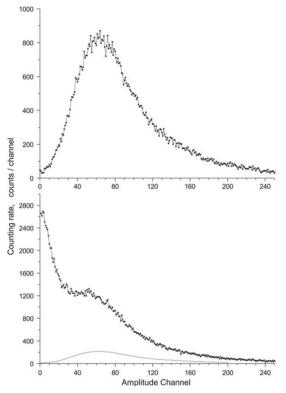
Figure 1. Amplitude distribution of the PMT pulses. (At the bottom with low noise, at the top the single electron distribution given by the subtraction of noise.) [5]
