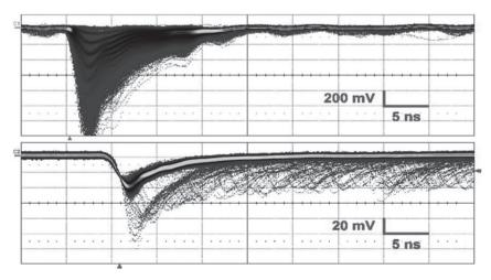
Figure 2. Oscilloscope view of pulses of avalanche photodiode matrix (M-APD). [5]
