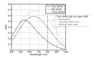
Figure 8. PDE of thick, thin and Red-Enhanced SPADs. [22]
