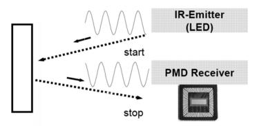
Figure 3. Working principle of the PDM time-of-flight camera. [3: 2]
