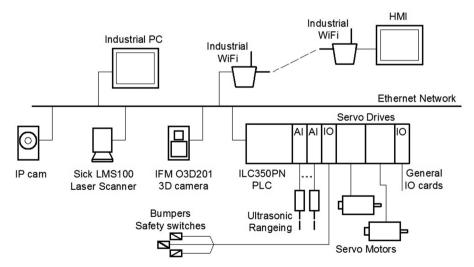
Figure 5. The structure of the advertising mobile robot platform. (Source: drawn by the author.)
