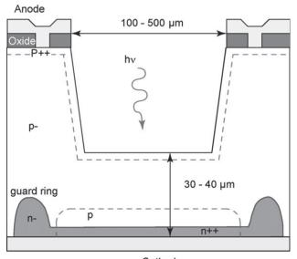
Cathode Figure 5. Cross-section of a thick SPAD. [4]
