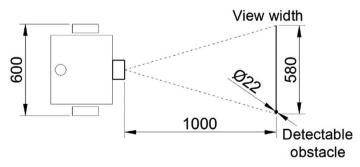
Figure 4. Detecting obstacles using O3D201. (Source: drawn by the author.)
