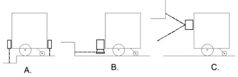
Figure 2. Typical obstacle types, and possible sensor solutions. (Source: drawn by the author.)
