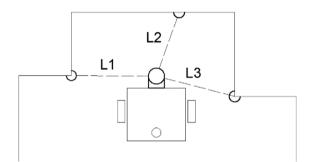
Figure 1. Indoor beacon based navigation measuring RSSI by detecting reflectors. (Source: drawn by the author.)
