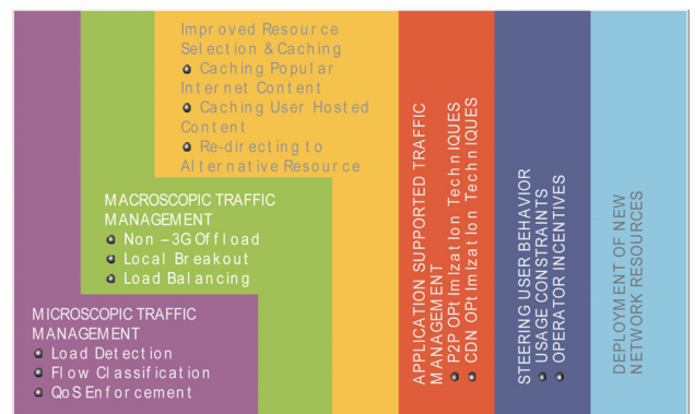
Fig. 3. Traffic management building blocks
