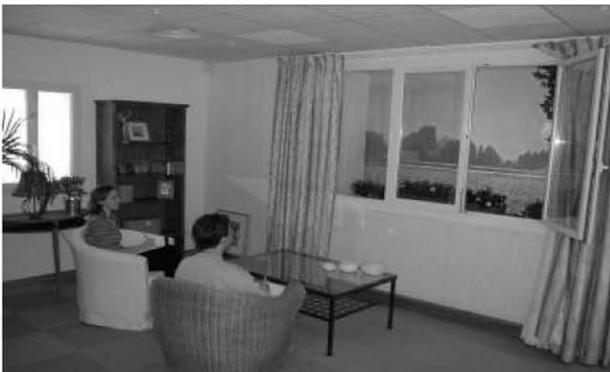
Fig. 6. Participants taking part in the laboratory studies. In being in home-like surroundings, aircraft flyovers are played back through loudspeakers. Participants do home-like activities like reading, discussing, and in addition also performance tests.
