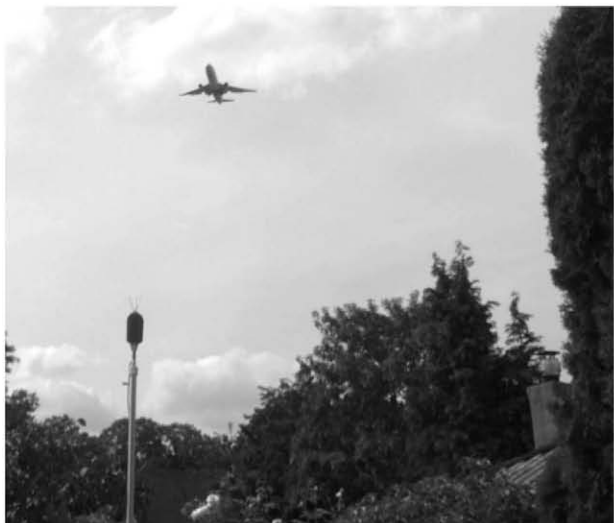
Fig. 7. In the unique approach of COSMA field studies, the "polluting" noise is directly measured outdoors at the location of participants, whereas the indoor noise level is computed from it through out/indoor transfer function measurements. (Note the microphone putted at 4m height on the left hand side of the picture.)
