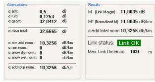
Fig. 13. Output of steady model for Sonabeam 52E.
