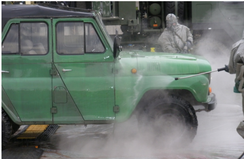
4. figure. The examination and technical test of DECOCONTAIN 3000 GDS system (source: authors)
