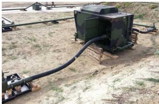
3. Figure. Fuel Pump for loading (Photo made by the author)
