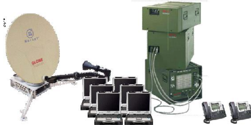
4. figure. MicroPoP system built-up [14]
