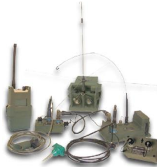
3. Figure. Components of REMBASS system a military UGS [14]
