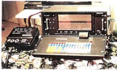
The IDEX ARPAD computer unit features a plasma display and can generate data for up to 18 guns. On-line surface meteorological data from a tripod-mounted automatic meteorological set at the battalion chief-of-staff's location can be factored into the calculations in real time. Visible left is the associated gun data display unit.
