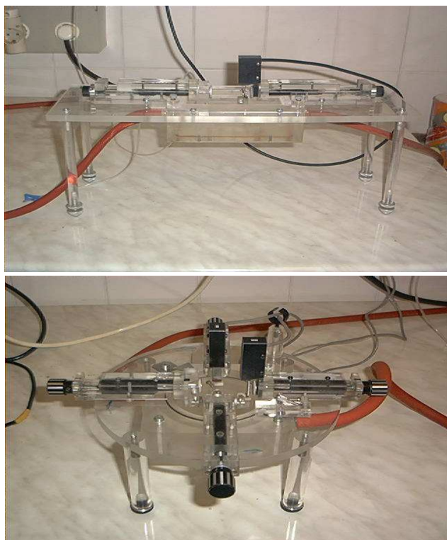
Figure 4. Uniaxial and biaxial laboratory test machines
