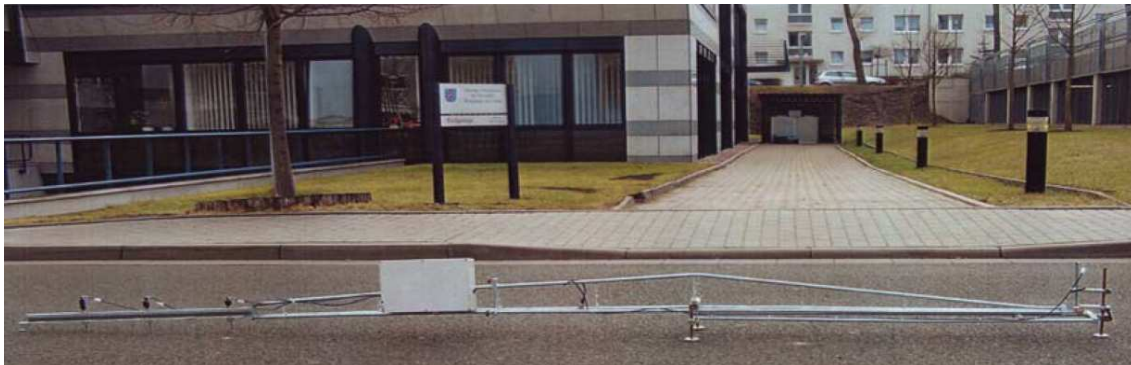
Figure 2. Automated Benkelman beam (Dähnert, 2005)
