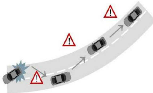
Figure 2. Inter-Vehicle Communication (Multi-Hop) [6]
