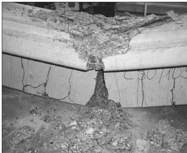
Fig. 2. Bending failure of the test FPT beam made of C90/105 grade concrete
