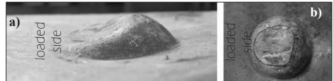
Fig. 7: Ultimate deformation of the embossment (a) side view (b) top view
