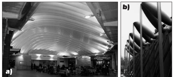
Fig. 27: a) Inflatable roof for Heathrow airport central bus station (architect: D5) (Lindstrand, 2006); b) 19.5 m x 40 m Exhibition Hall with air-inflated elements (architect: Festo AG & Co) in Germany (Festo)
