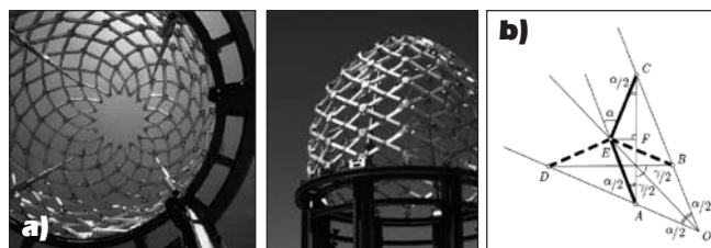
Fig.14: a) Iris dome by Hoberman, EXPO 2000 (Whitehead, 2000); b) angulated element (Jensen, Pellegrino, 2004)
