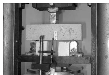
Fig. 14: Bending test of a notched beam, measure 70×70×250 mm, span: 180 mm
