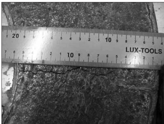
Fig. 8: Crack through the specimen
