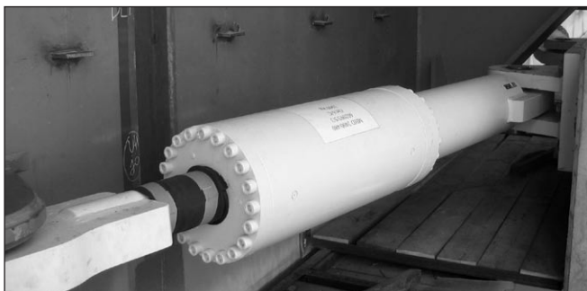
Fig. 9: Longitudinally positioned horizontal hydraulic support
