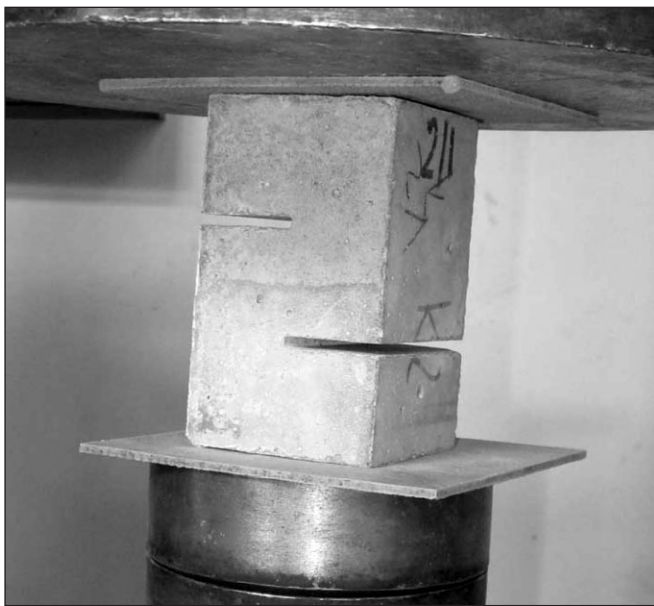
Fig. 16: Shear test of a 70x70 mm excised block
