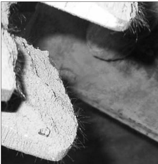
Fig. 3: Well mixed fibres in concrete before adding water
