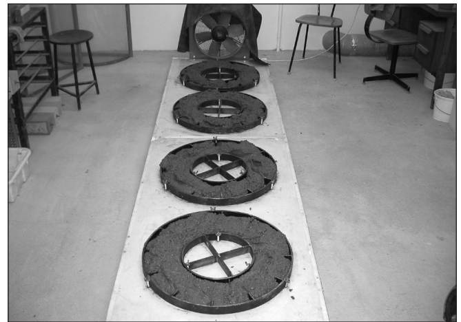
Fig. 2: Wind tunnel with four formworks after compacting concrete
