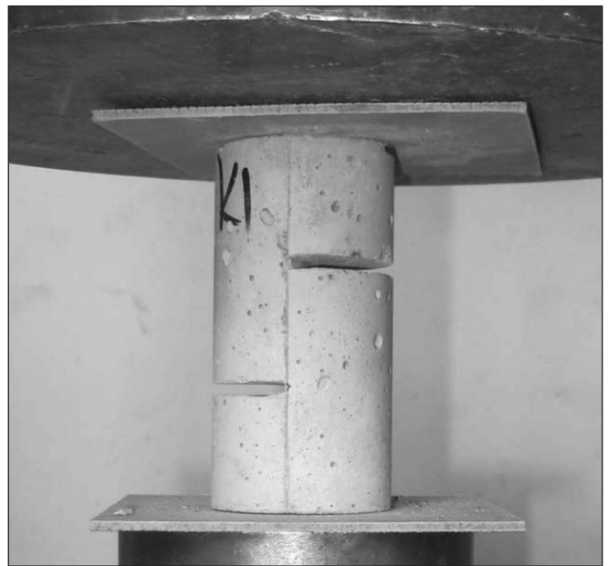
Fig. 18: Shear test of a notched cylinder, diameter 60 mm
