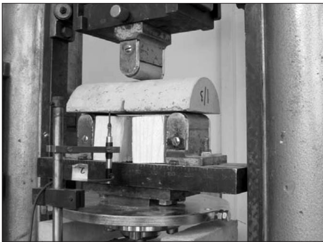
Fig. 15: Bending test of a notched, halved cylinder, diameter 100 mm, span: 150 mm
