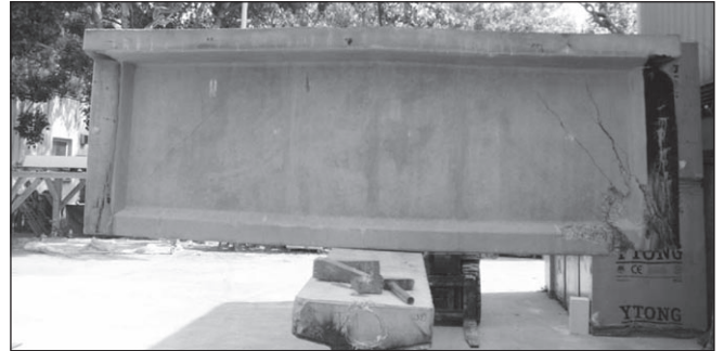
Fig. 13: Beam with Mix 4 after failure concrete (Mix 1) after failure
