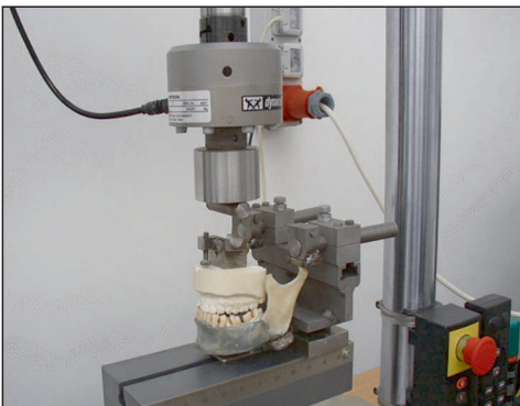
Figure 5. Investigation of a mandible with photoelastic coating technique
