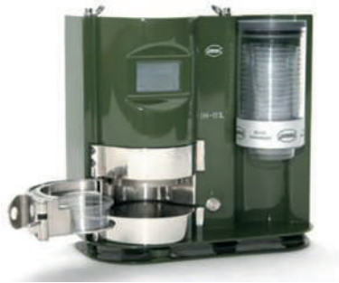
Figure 6. IH-111L Portable radiological measuring instrument
