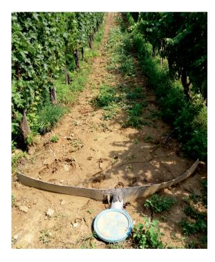
Photo 2. Sediment trap with eroded material on 26 May 2018 (Photo by Dezső, J.)
