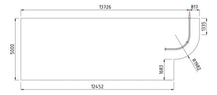
Figure 3. *The size of the area around the connection of the output manifold of the water source.* [Created by the author.]
