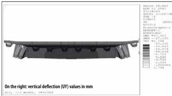
Fig. 5 Deformed shape at load P = 120 kN (magnified 10 times)
