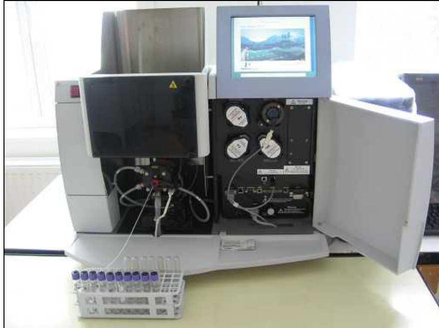
Figure 1: Perkin-Elmer atomic absorption spectroscopy A Analyst 200
