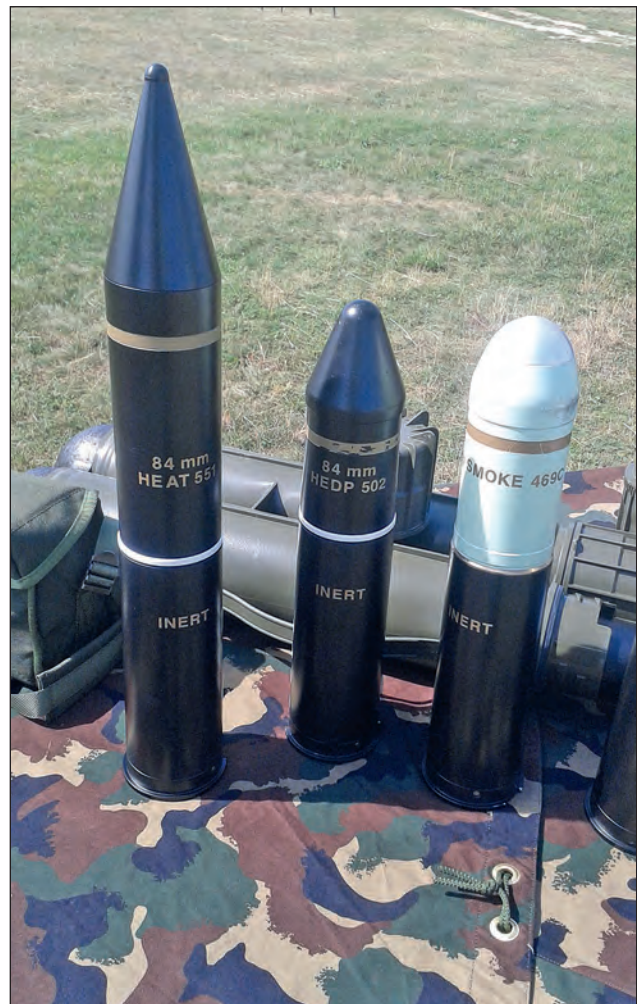
Figure 3. Different kinds of ammunitions of the Carl-Gustaf M4 recoilless weapon depending on tasks
