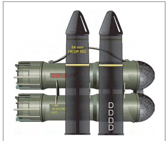
Figure 12. The 84 mm HEDP 502 ammunition for urban environment
