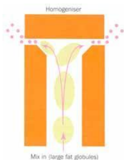
Fig 3(a) Schematic diagram of homogenisation showing the break up of large fat globules into small droplets
