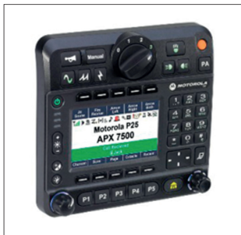
Figure 6: Motorola Integrated Control Panel 23
