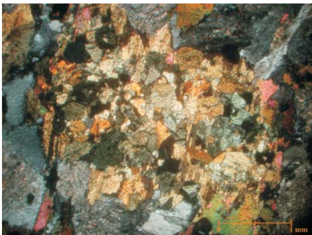
Figure 4. Amphibole aggregate in mafic enclave. (Üh-37, 175.9 m) Small grains of amphibole form aggregate. ×N
