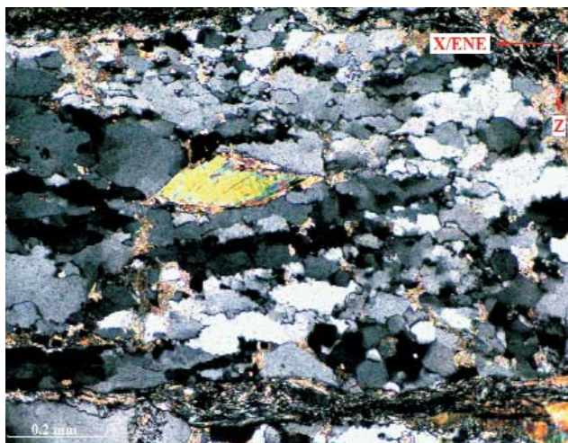
Figure 5. Microfabric detail from a well-foliated monzogranite (Üh-29, 111.9 m)
